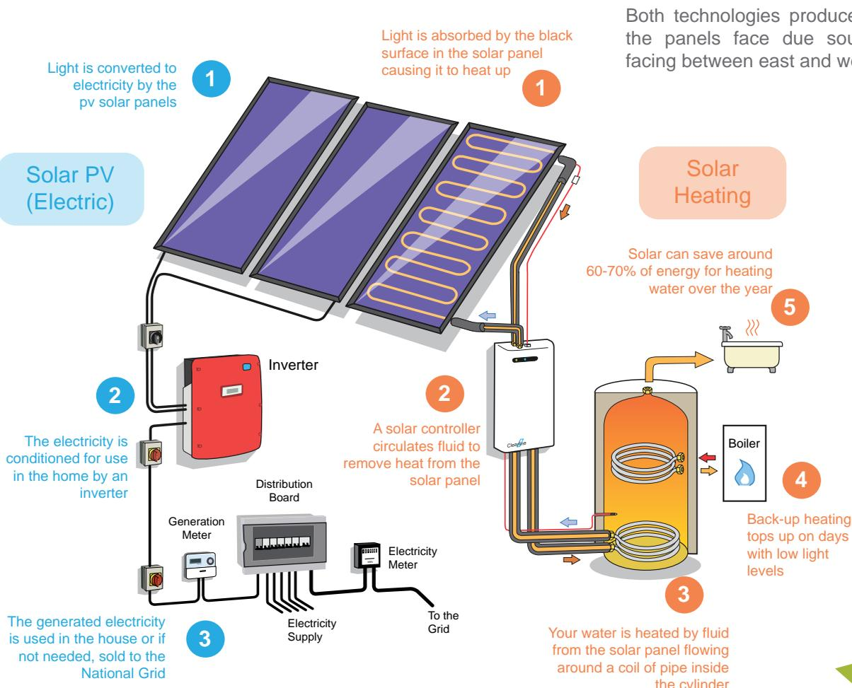
Both technologies produce most energy when the panels face due south, but installations facing between east and west are also effective.
