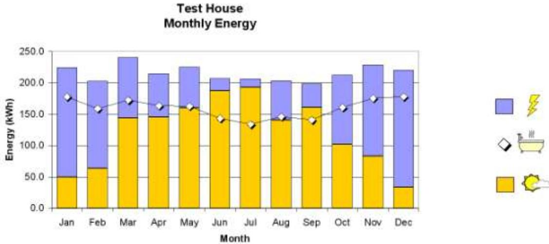
It can be seen that the solar energy (orange) follows a characteristic solar curve with the solar heating system making most of its contribution to hot water demand during the summer, spring and autumn.
